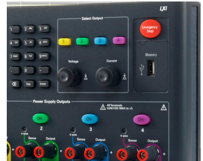
Figure 11. The N6705's front panel USB port.
