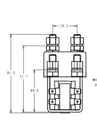
The contactors can be mounted either horizontally or vertically If mounted vertically the contact studs must point upwards with the exception of the JAB and it's derivatives which should be mounted with the contact studs pointing down
