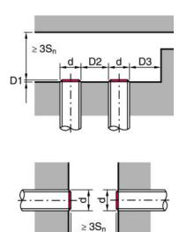
S<sub>n</sub> [mm] D1 [mm] D2 [mm] 2 18 D3 [mm] 6
