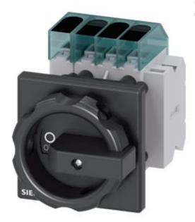
Switch disconnector 3LD3, main switch 3-polig + N, lu 25A operational switch at AC-23 A at 400 V 9,0 kW front mounted Base mounting with center-hole 22,5 mm knob-operated mechanism black  $66 \times 66$  mm with auxiliary 1NO+1NC
