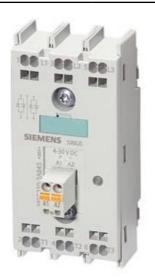
SOLID STATE RELAY 3-PHASE 3RF2 55 A 40 DEG. C 48-600 V / 4-30 V DC 2PH.-CONTROLLED SPRING-TYPE TERMINAL BLOCKING VOLTAGE 1200 V
