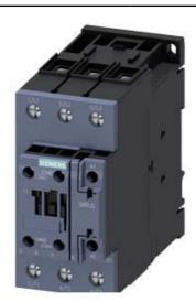
CONTACTOR,AC3:22KW/400V, 1NO+1NC, 110V AC 50HZ, 3-POLE, SIZE S2, SCREW TERMINAL UPRIGHT MOUNTING POSITION
