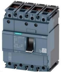
CIRCUIT BREAKER 3VA1 IEC FRAME 160 BREAKING CAPACITY CLASS S ICU=36KA @ 415 V 4-POLE, LINE PROTECTION TM210, FTFM, IN=100A OVERLOAD PROTECTION IR=100A FIXED SHORT CIRCUIT PROTECTION II=10 X IN NEUTRAL PROTECTION 100% BUSBAR CONNECTION
