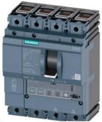
CIRCUIT BREAKER 3VA2 IEC FRAME 100 BREAKING CAPACITY CLASS L ICU=150KA @ 415 V 4POLE, LINE PROTECTION ETU330, LIG, IN=100A OVERLOAD PROTECTION IR=40A ...100A SHORT CIRCUIT PROTECTION II=1,5...12 X IN NEUTRAL PROTECTION ADJUSTABLE(OFF,50%,100%) GROUNDFAULTPROTECTION IG=0,2... 1 X IN, TG=0,1/0,3MS CABLE CONNECTION
