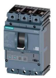
CIRCUIT BREAKER 3VA2 IEC FRAME 100 BREAKING CAPACITY CLASS L ICU=150KA @ 415 V 3POLE, LINE PROTECTION ETU330, LIG, IN=63A OVERLOAD PROTECTION IR=25A ...63A SHORT CIRCUIT PROTECTION II=1,5...12 X IN GROUNDFAULTPROTECTION IG=0,2... 1 X IN, TG=0,1/0,3MS BUSBAR CONNECTION
