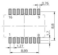
Unless otherwise defined tolerance: ±0,10mm no vias or traces underneath the component
