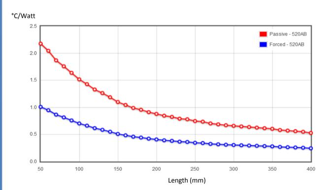
Thermal Resistance is calculated based on a distributed heat load and vertically mounted fins anodised heatsink with a 60°C temperature.
