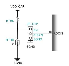
Figure 11. OTP Schematic Circuit
