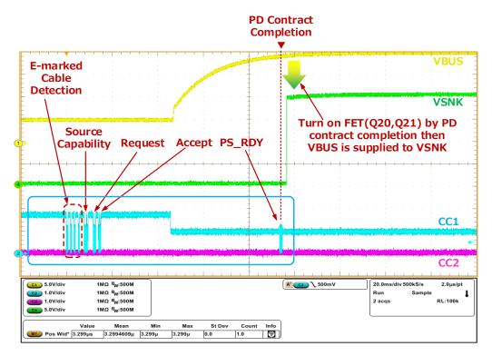
Figure 17. The Waveform of the USB PD Negotiation at 20V (Detailed PD Communication)
