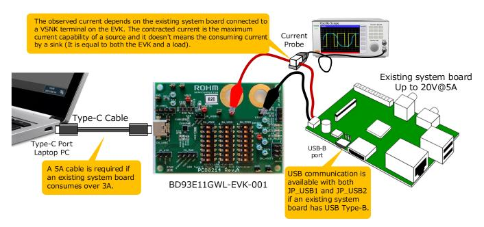
Figure 6. An example of the connection of the EVK supplying power to an existing system board
