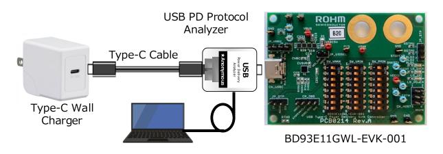
Figure 8. An example of the connection with a protocol analyzer for PD communication
