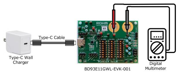
Figure 4. An evaluation for only EVK with Type-C cable
