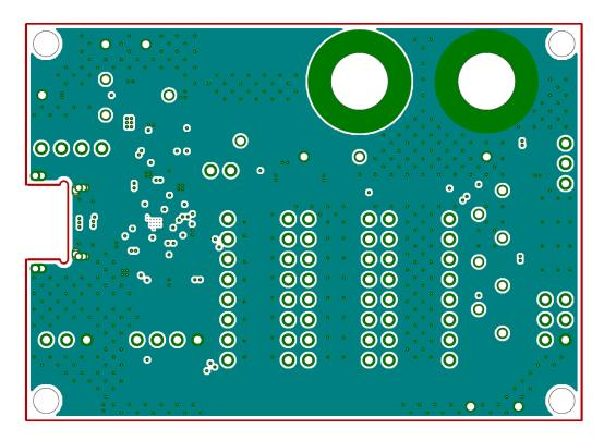
Figure 13. Middle Layer 1 (Top View)
