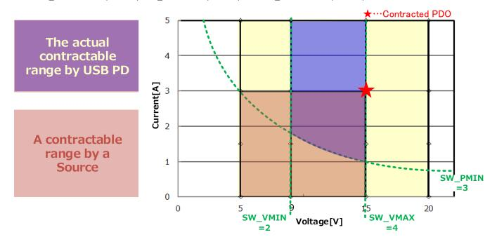
Figure 10. The contractable range with a source under the example
