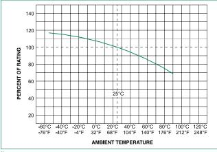
Note: 1. Rerating depicted in this curve is in addition to the standard derating of 25% for continuous operation.
