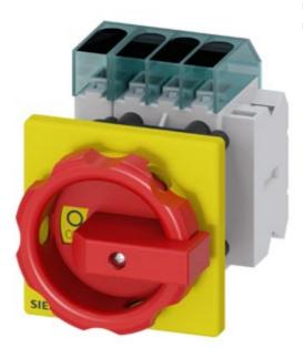
Switch disconnector 3LD3, main switch 3-polig + N, lu 16A operational switch at AC-23 A at 400 V 7,5 kW front mounted Base mounting with center-hole 22,5 mm rotary operationg mechanism red/yellow 66 x66 mm with auxiliary 1NO+1NC
