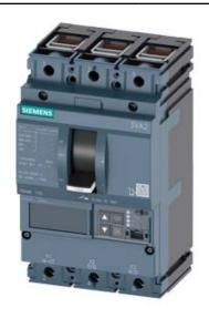
CIRCUIT BREAKER 3VA2 IEC FRAME 100 BREAKING CAPACITY CLASS M ICU=55KA @ 415 V 3POLE, LINE PROTECTION ETU560, LSIG, IN=63A OVERLOAD PROTECTION IR=25A ...63A SHORT CIRCUIT PROTECTION ISD=0,6..10X IN, II=1,5...12X IN NEUTRAL PROTECTION OPTIONAL WITH EXT. CT,UPTO 160% GROUNDFAULT, SWITCHABLE IG=0,2... 1 X IN, TG=0,050,8MS CABLE CONNECTION
