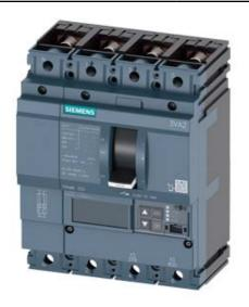
CIRCUIT BREAKER 3VA2 IEC FRAME 250 BREAKING CAPACITY CLASS L ICU=150KA @ 415 V 4POLE, LINE PROTECTION ETU860, LSIG, IN=250A OVERLOAD PROTECTION IR=100A ...250A SHORT CIRCUIT PROTECTION ISD=0,6..10X IN, II=1,5..10X IN NEUTRAL PROTECTION ADJUSTABLE (OFF, UPTO 100%) GROUNDFAULT, SWITCHABLE IG=0,2... 1 X IN, TG=0,050,8MS BUSBAR CONNECTION
