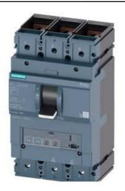
CIRCUIT BREAKER 3VA2 IEC FRAME 630 BREAKING CAPACITY CLASS M ICU=55KA @ 415 V 3-POLE, LINE PROTECTION ETU350, LSI, IN=400A OVERLOAD PROTECTION IR=160A ...400A SHORT CIRCUIT PROTECTION ISD=1,5... 10 X IR, II=12 X IN BUSBAR CONNECTION
