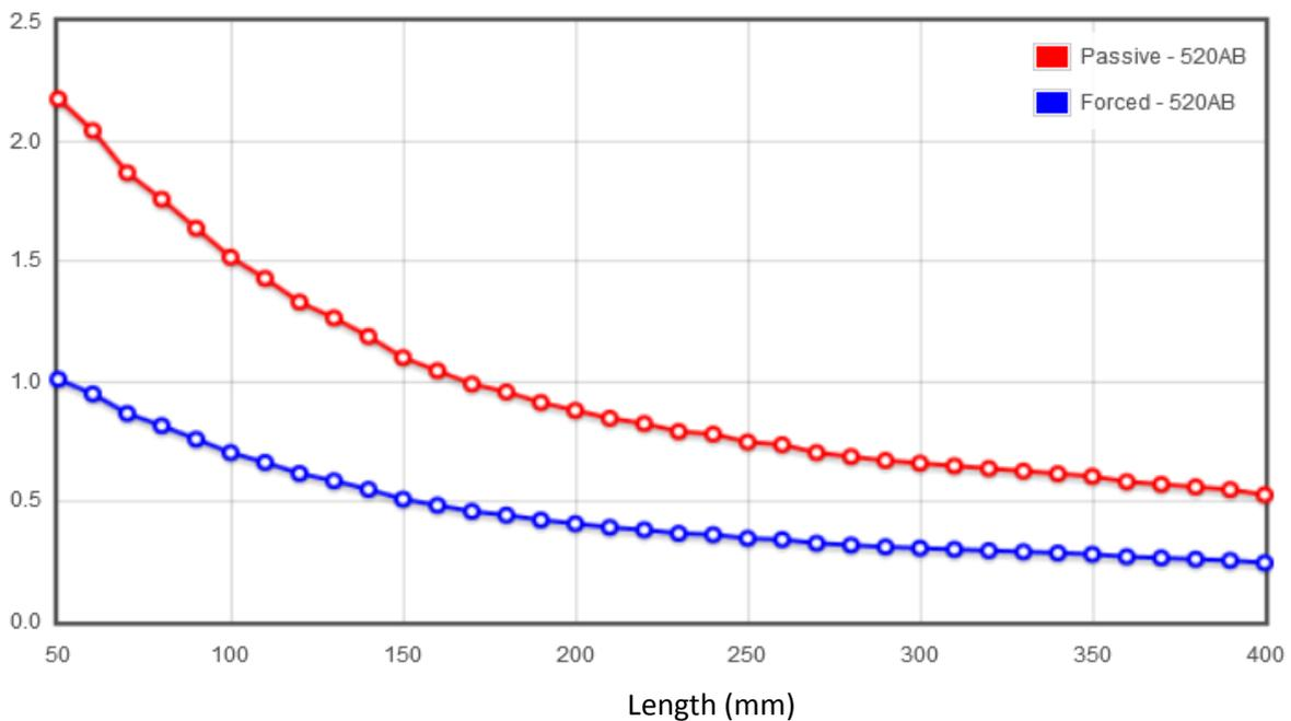
Thermal Resistance is calculated based on a distributed heat load and vertically mounted fins anodised heatsink with a 60°C temperature.
