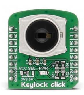
**Keylock click** carries a processed sealed key lock mechanism that can be set in three different positions. The click is designed to run on either 3.3V or 5V power supply. It communicates with the target microcontroller over the PWM, INT, and AN pin on the mikroBUS $^{\text{TM}}$  line.
