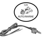
Rated at 6 amps at 12-14 VDC, this ON-OFF SPST switch could easily be used for any number of appliances, as well as for arming alarms. Included is a miniature escutcheon plate with the legends ON and OFF. Mount hole: 1/4" diameter round.
