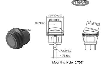
Current Rating: 20A-12VDC Contact Resistance: 50m Ohm max DC 500V 100m Ohm min. Insulation Resistance: Dielectric Strength: AC 1500V for 1 minute **Body Material:** Nylon 66 (94V-2) Actuator Material: PC (94-V2), with black silicone cover Terminal Material: Silver plated, Copper Alloy .187" Quick Connect Terminal Type:
