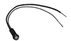
12-14 Volt LED Panel Lamp for .25" hole size. This series has typical LED (T1-3/4") Size. Lead wires are 6" long, stripped .380" on ends (red and black insulation indicates polarity).
