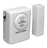
Provides an electronic "ding-dong" to announce someone entering a door. This may be the least expensive door annunciator, and the most easily installed. Attach the magnet to your door and sounding device to the door frame (or vice versa), if you like. Double sticky foam tape makes mounting quick work. A sophisticated sound announces the entry of a customer each time the door is opened.
