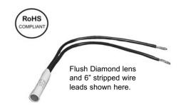
Long Life, Solid State, light emitting diodes make this series of snap-in lamps a very dependable component. Available in popular voltages as well as the standard LED voltage (2 Volt series); use Ohm's law to calculate a series resistor if other voltages are needed. All LED'S on this page operate at 20 mA DC typical.
