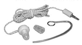
This molded white earphone has 15 ohm impedance. Unitary construction eliminates need for a detachable earpiece. Miniature (1/8" D) plug termination. Used widely in hospitals and other institutions.
