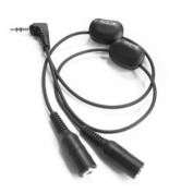
3.5mm Stereo Plug to (2) 3.5mm Stereo Jacks with 10" cords. Each 3.5mm stereo jack has in-line volume control to control audio output on each jack.
