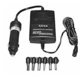
Designed to power battery operated equipment drawing up to 1 amp. current (1000mA). Completely regulated and maintains voltage constant within 1 Volt despite wide variations in load current. Accepts 12-16VDC input from conventional negative ground.
