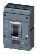
Circuit breaker 3VA6 UL Frame 800 breaking capacity class M 35kA @ 480 V 3-pole, Line protection ETU856, LSI, In=600A overload protection, 100% rated Ir=240A ...600A Short-circuit protection Isd=0.6..12x In, Ii=1.5..12x In N conductor protection optionally with external CT up to 160% Ground-fault alarm message via EFB300 or COM
