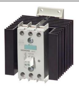
SEMI-CONDUCTOR CONTAC.3-PH.3RF2 AC51 20A 40 DEG. C 48-600V / 230V AC 3-PHASE CONTROLLED SCREW TERMINAL BLOCKING VOLTAGE 1200V
