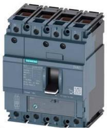
CIRCUIT BREAKER 3VA1 IEC FRAME 160 BREAKING CAPACITY CLASS S ICU=36KA @ 415 V 4-POLE, LINE PROTECTION TM220, ATFM, IN=100A OVERLOAD PROTECTION IR=70A ...100A SHORT CIRCUIT PROTECTION II=10 X IN NEUTRAL PROTECTION 100% CABLE CONNECTION
