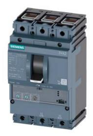
CIRCUIT BREAKER 3VA2 IEC FRAME 160 BREAKING CAPACITY CLASS C ICU=110KA @ 415 V 3POLE, LINE PROTECTION ETU320, LI, IN=100A OVERLOAD PROTECTION IR=40A ...100A SHORT CIRCUIT PROTECTION II=12 X IN CABLE CONNECTION
