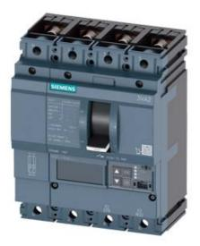
CIRCUIT BREAKER 3VA2 IEC FRAME 160 BREAKING CAPACITY CLASS C ICU=110KA @ 415 V 4POLE, LINE PROTECTION ETU850, LSI, IN=40A OVERLOAD PROTECTION IR=16A ...40A SHORT CIRCUIT PROTECTION ISD=0,6..10X IN, II=1,5..12X IN NEUTRAL PROTECTION ADJUSTABLE (OFF, UPTO 160%) BUSBAR CONNECTION
