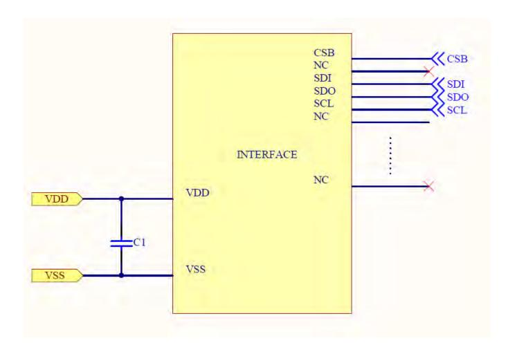
Pin connected to MCU interface: CSB,SDI,SDO,SCL
