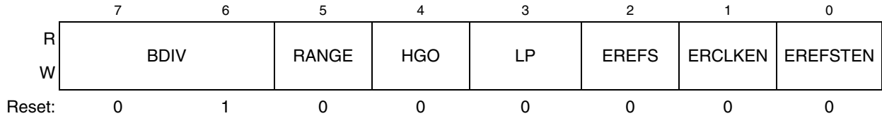
Figure 11-4. ICS Control Register 2 (ICSC2)
