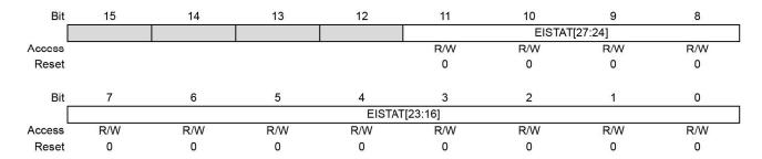
Bits 11:0 - EISTAT[27:16] Early Interrupt Status for Corresponding Analog Input bits
