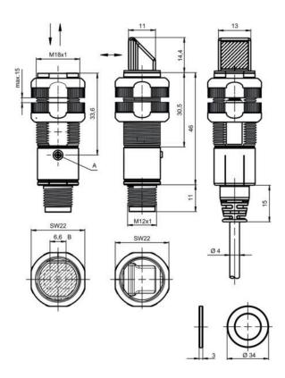
B Optical axis A Indicator diode
