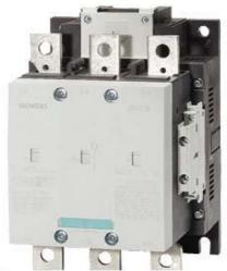
VAC. CONTACTOR, 132KW/400V/AC-3 AC(40...60HZ)/DC OPERATION UC 110-127V AUXILIARY CONTACTS 2NO+2NC 3-POLE, SIZE S10 BAR CONNECTIONS CONVENT. OPERATING MECHANISM
