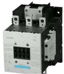
CONTACTOR, 275A/AC-1, AC(40...60HZ)/DC OPERATION UC 42...48V AUXIL. CONTACTS 2NO+2NC 3-POLE, SIZE S6 BAR CONNECTIONS CONVENT. OPERATING MECHANISM
