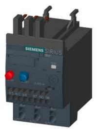
OVERLOAD RELAY 0.55...0.80 A FOR MOTOR PROTECTION SZ S00, CLASS 10, F. MOUNTING ONTO CONTACTOR MAIN CIRCUIT: SPRING TERMINAL AUX. CIRCUIT: SPRING TERMINAL MANUAL-AUTOMATIC-RESET
