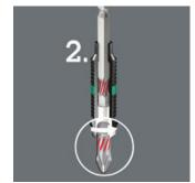
Higher peak loads are minimised through the torsion effect of the bit shaft (Phase 2). This effect is achieved with a specific heat treatment after the hardening process of the bits. This reduces the hardness of the shaft in comparison to the drive tip.
