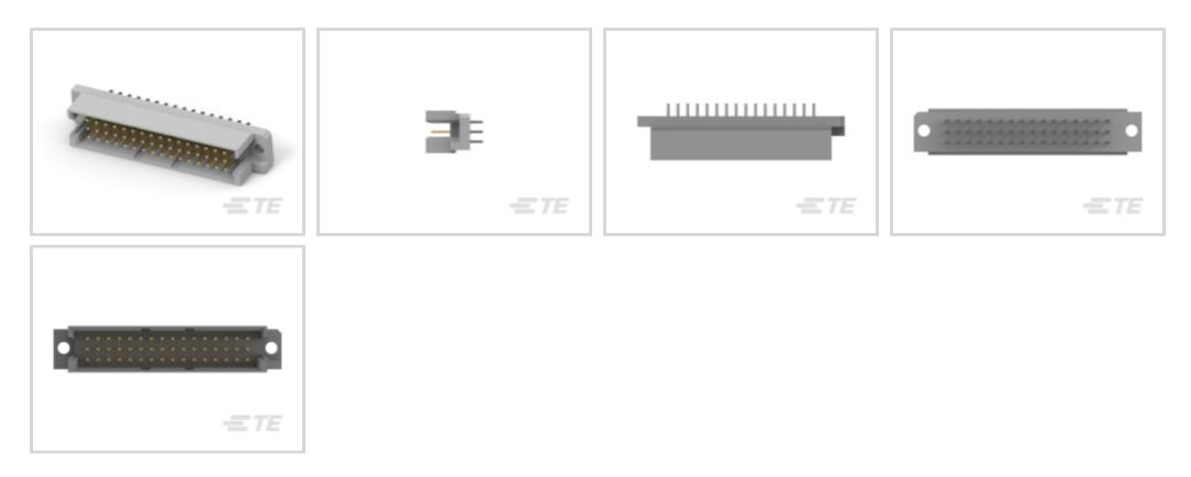
Connector & Housing Type: Plug Connector System: Board-to-Board Termination Post & Tail Length: 3.3 mm [.13 in] Number of Positions: 48 Centerline (Pitch): 2.54 mm [.1 in]
