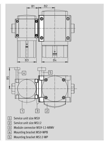
The larger mounting bracket must always be used on the module connector. The mounting bracket
