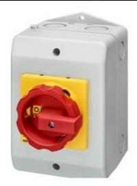
EMERG. STOP SWITCH 4-POLE IU=25, P/AC-23A AT 400V=9.5KW 1 N-TERMINAL INSULATION-ENCLOSED, IP65 ROTARY ACTUATOR RED/YELLOW (EMERG. STOP) METRIC SCREW CONNECTION
