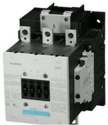
CONTACTOR, 275A/AC-1, AC(40...60HZ)/DC OPERATION UC 240...277V AUXIL. CONTACTS 2NO+2NC 3-POLE, SIZE S6 BAR CONNECTIONS CONVENT. OPERATING MECHANISM
