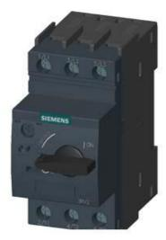
SPECIAL TYPE CIRCUIT BREAKER SIZE S00, FOR TRANSFORMER PROTECTION A-RELEASE 10...16A, SHORT-CIRCUIT RELEASE 286A, SCREW TERMINAL, STANDARD SWITCHING CAPACITY AMBIENT TEMPERATURE -50 DEGREES C 500 SWITCHING CYCLES
