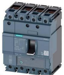
CIRCUIT BREAKER 3VA1 IEC FRAME 160 BREAKING CAPACITY CLASS S ICU=36KA @ 415 V 4-POLE, LINE PROTECTION TM220, ATFM, IN=40A OVERLOAD PROTECTION IR=28A ...40A SHORT CIRCUIT PROTECTION II=10 X IN NEUTRAL PROTECTION 100% CABLE CONNECTION
