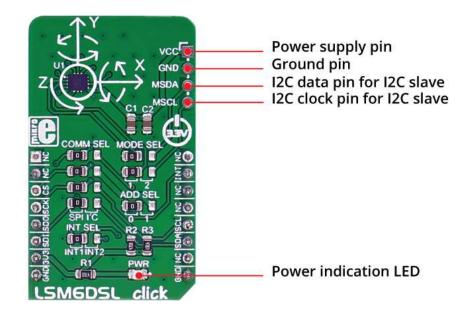
Mode 1: I2C slave interface or SPI serial interface is available.
