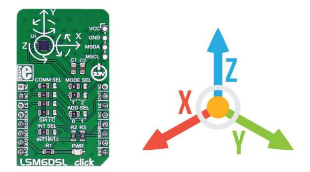
The event-detection interrupts enable efficient and reliable motion tracking and contextual awareness, implementing hardware recognition of free-fall events, 6D orientation, click and double-click sensing, activity or inactivity, and wakeup events
