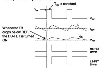
Figure 2—Heavy Load Operation
