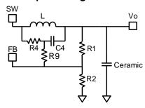
Figure 10—Simplified Circuit of Ceramic Capacitor
