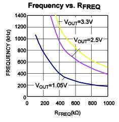
Generally, the NB638 is set for 200 kHz to 1MHz application. It is optimized to operate at high switching frequency with high efficiency. High switching frequency makes it possible to utilize small sized LC filter components to save system PCB space.
