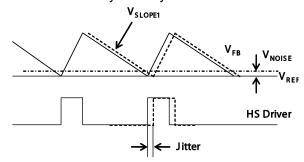
Figure 4—Jitter in PWM Mode
