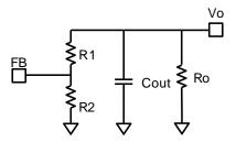
Figure 8—Simplified Circuit in skip Mode
