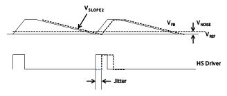
Figure 5—Jitter in Skip Mode
