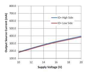
Figure 16. Output Source Current vs. Supply Voltage
