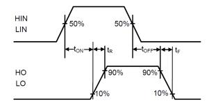
Figure 1. Input / Output Timing Diagram
