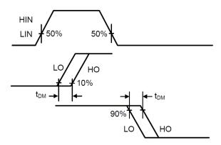
Figure 3. Delay Matching Waveform Definitions
