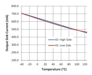
Figure 19. Output Sink Current vs. Temperature
