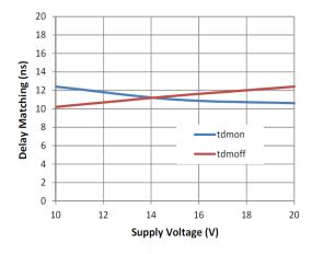
Figure 14. Delay Matching vs. Supply Voltage
