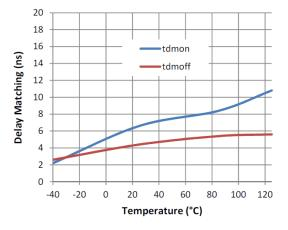
Figure 15. Delay Matching vs. Temperature
