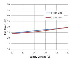
Figure 10. Fall Time vs. Supply Voltage
