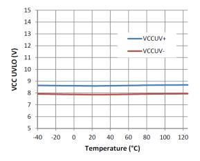
**Figure 24.** V<sub>CC</sub> UVLO vs. Temperature
