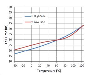
Figure 11. Fall Time vs. Temperature
