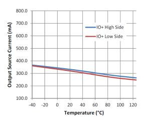
Figure 17. Output Source Current vs. Temperature
