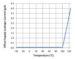
Figure 25. Offset Supply Leakage Current Temperature
