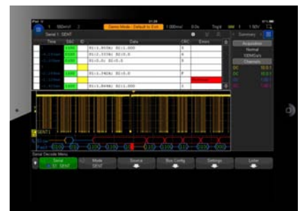
Figure 8. Remotely control the 3000T X-Series via tablet device.
