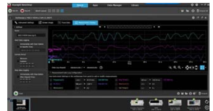
Figure 4. Use BenchVue for remotely logging and plotting measurement data.
