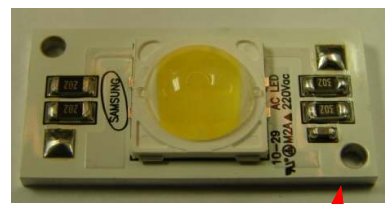
Temperature measurement point
