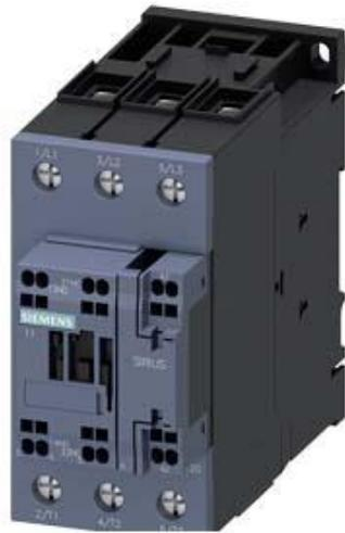
SCHUETZ,AC3:30KW/400V, 1S+1OE, AC/DC 175-280V, M. VARISTOR, 3POL, BGR. S2, FEDERZUGANSCHLUSS
