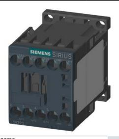
COUPLING RELAY, AC-3, 3KW/400V, 1NO, DC 24V, 0.7...1.25\*US, 3-POLE, SZ S00 SCREW TERMINAL
