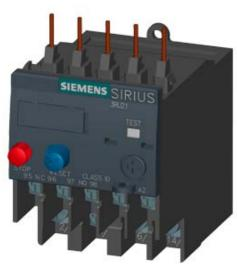
OVERLOAD RELAY 0.14...0.20 A FOR MOTOR PROTECTION SZ S00, CLASS 10, F. MOUNTING ONTO CONTACTOR MAIN CIRCUIT: RING CABLE LUG AUX. CIRCUIT: RING CABLE LUG MANUAL-AUTOMATIC-RESET
