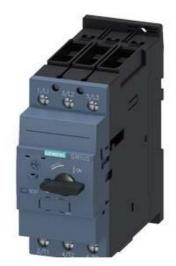
CIRCUIT BREAKER, SIZE S2, FOR MOTOR PROTECTION, CLASS 20, A-RELEASE 14...20A, N-RELEASE 260A, SCREW TERMINAL, STANDARD BREAKING CAPACITY
