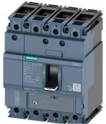
CIRCUIT BREAKER 3VA1 IEC FRAME 160 BREAKING CAPACITY CLASS M ICU=55KA @ 415 V 4-POLE, LINE PROTECTION TM220, ATFM, IN=160A OVERLOAD PROTECTION IR=112A ...160A SHORT CIRCUIT PROTECTION II=10 X IN NEUTRAL UNPROTECTED BUSBAR CONNECTION
