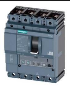
CIRCUIT BREAKER 3VA2 IEC FRAME 160 BREAKING CAPACITY CLASS M ICU=55KA @ 415 V 4POLE, LINE PROTECTION ETU330, LIG, IN=160A OVERLOAD PROTECTION IR=64A ...160A SHORT CIRCUIT PROTECTION II=1,5...10 X IN NEUTRAL PROTECTION ADJUSTABLE(OFF,50%,100%) GROUNDFAULTPROTECTION IG=0,2... 1 X IN, TG=0,1/0,3MS BUSBAR CONNECTION
